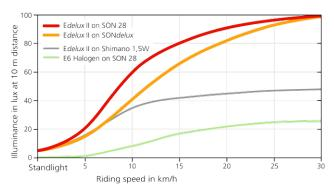
In contrast to mere 6 Volt 1.5 Watt hubs power output is not reduced at high speed. At high riding speed, when good visibility is vital, you will enjoy unlimited maximum illumination; using an Edelux II with up to 100 lux. So SONdelux will be first choice for everyone who prefers minimum weight (385 g), extremely smooth running plus a lot of Illumination at high riding speed.
