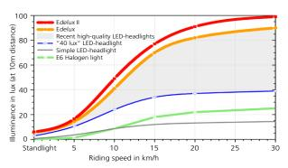
High illuminance is vital at poor viewing conditions (wet road surface, blinding oncoming traffic). Highest illuminance should be projected at the upper edge of the light beam to create a good visibility at far distance.
