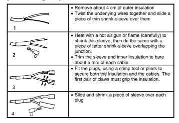
Headlamps with integrated switch by other manufacturers (e.g. Lumotec oval senso plus) are usually equipped with twin cables instead of coaxial cable. Instead of step 1 and 2 the cable only has to be cut to length, the two wires separated for about 3 cm and the insulation removed at about 5 mm.
