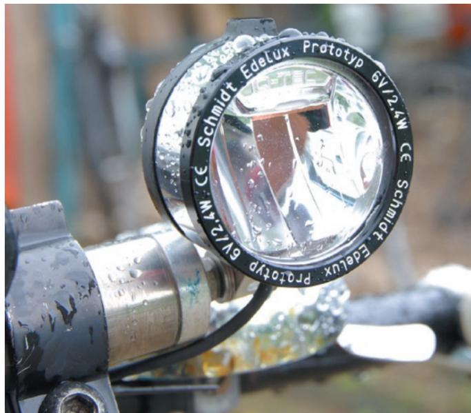
for waterproofing. The switch (for auto, on, off modes) is a black plastic ring which slides around a groove in the body, with a magnet operating an internal reed switch – so no openings to let in moisture. The engraved black ring around the
